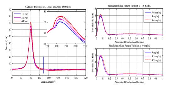
Figure 3. (a) measured and predicted cylinder pressure at different load (b) predicted heat release at different amount of fuel injected
