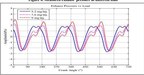
Figure 4. Measured exhaust pressure at different load
