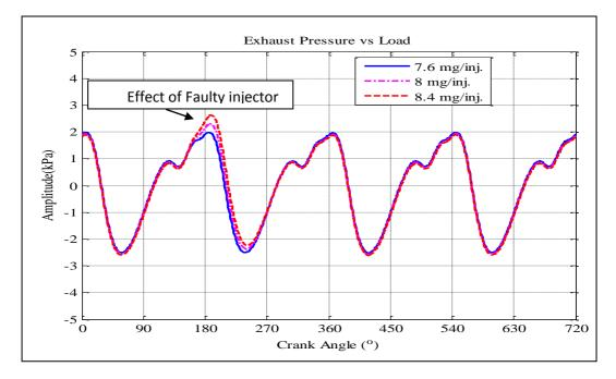
Figure 8. Predicted exhaust pressure with injector fault at cylinder 1 at low load
