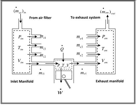
Figure 1 Schematic diagram of a 4 cylinder diesel engine, (subscript 1 refers to cylinder 1, etc)
