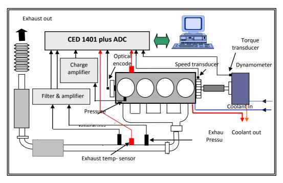
Figure 2. Schematic diagram of engine and measurement equipments
