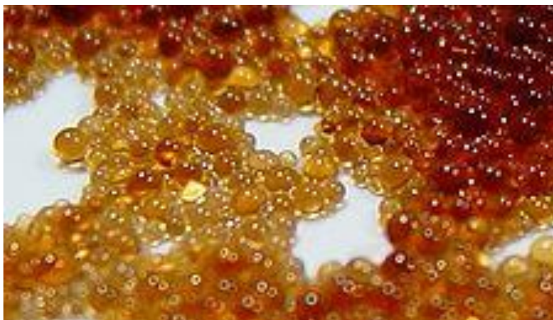
Fig. 1 Ion exchange resin beads [7].
