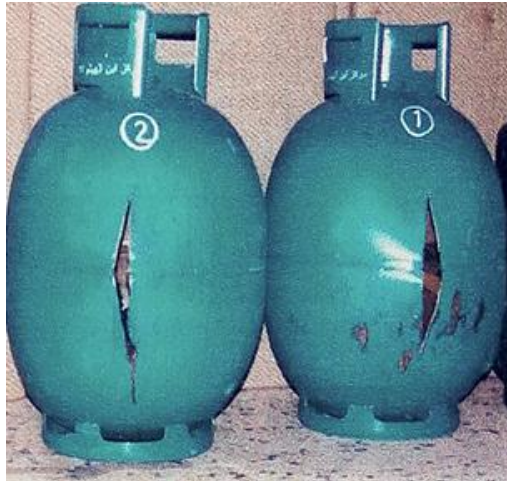
Fig.3. Failure Locations of the cylinders.
