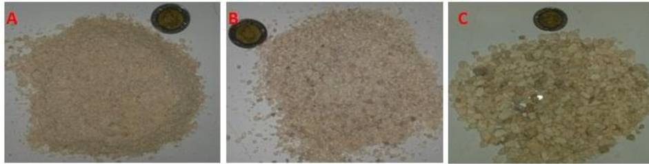
Fig.8: Photographs showing the three aggregate sizes in the Al Abyar quarry. (A) Fine aggregates, (B) Medium aggregates, and (C) Coarse aggregates.
