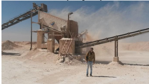
Fig. 6: Field image showing the second stage (i.e. crushed of raw material) in the Al Abyar quarry.
