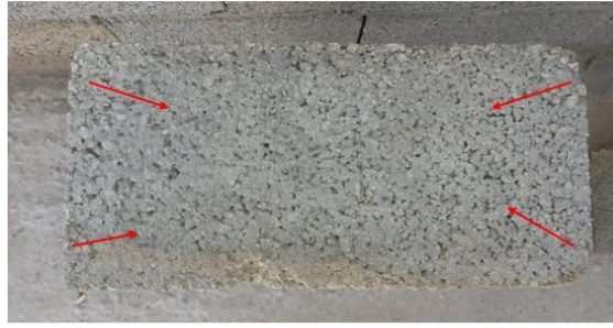
Fig. 11: Photograph showing fine aggregates filling the spaces between aggregates in a dimension stones the Al Abyar quarry.
