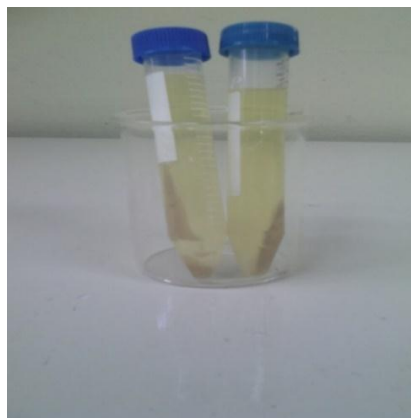
Figure 2: The supernatant and residue after the centrifugation of fenugreek seed powder and distilled water mixture.
