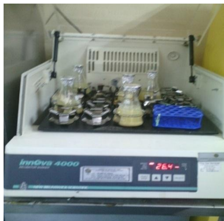
Figure 1: Fenugreek seed powder mixed with distilled water in 250mL glass flasks and continuously agitated by the shaker for 24 hours at room temperature.
