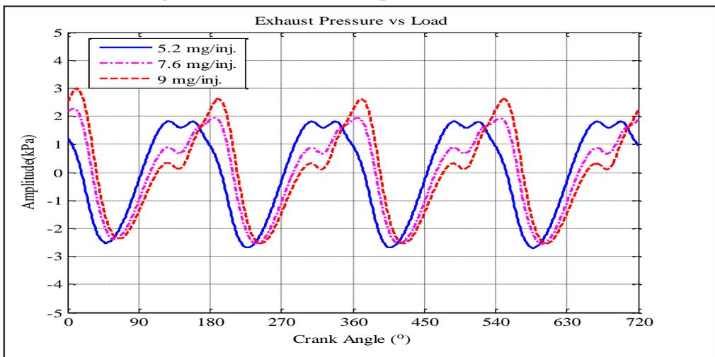
Figure 5. Predicted exhaust pressure as function of injected fuel (load)
