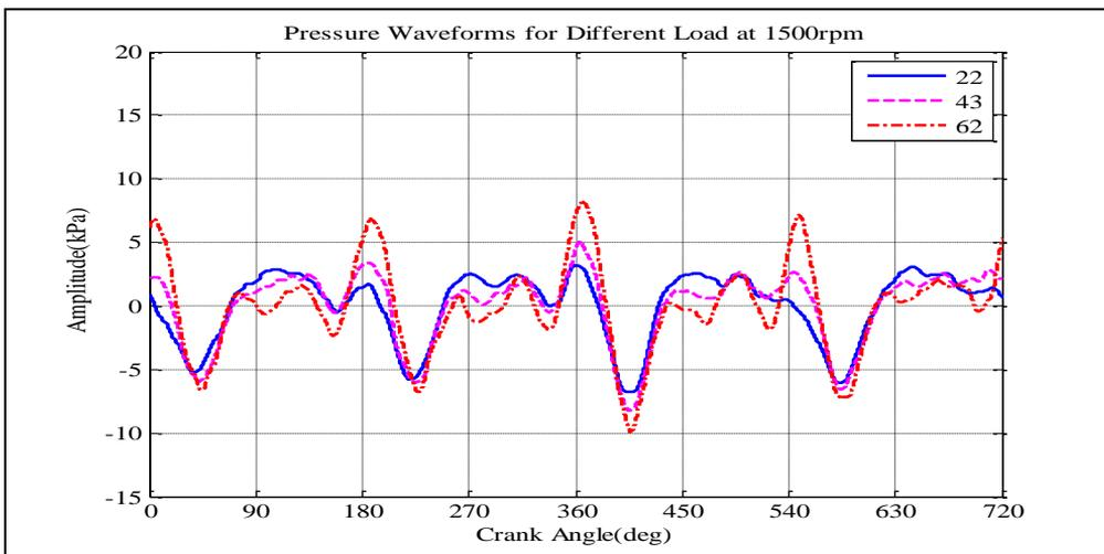
Figure 4. Measured exhaust pressure at different load
