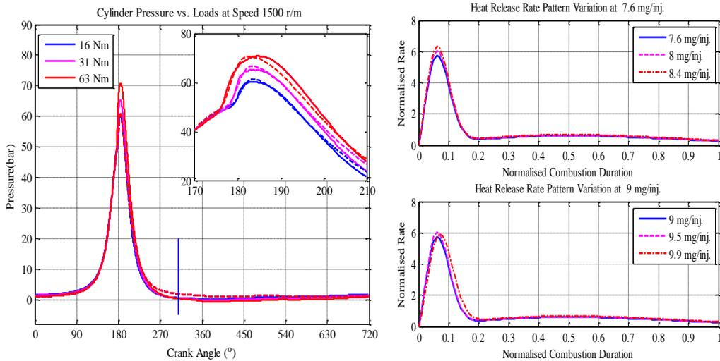
**Figure 3. (a) measured and predicted cylinder pressure at different load (b) predicted heat release at different amount of fuel injected**
