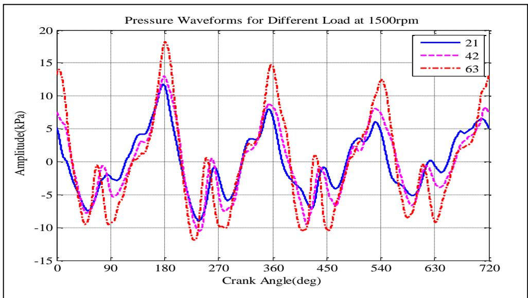
Figure 6. Measured exhaust pressure with injection faults at cylinder 1
