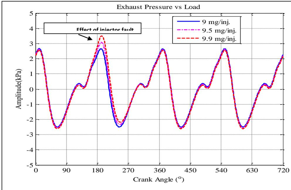
Figure 7. Predicted exhaust pressure with injector fault at cylinder 1 at high load
