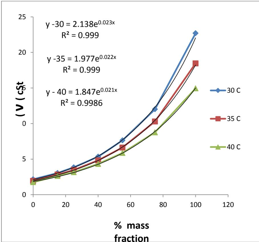
Figure (2) kinematic viscosity at different temperatures vs percentage of blends.
