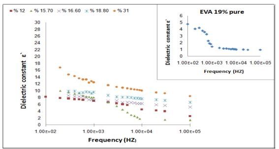
Figure(1): The frequency dependence of dielectric constant for the pure EVA and its composites (with PPy)
