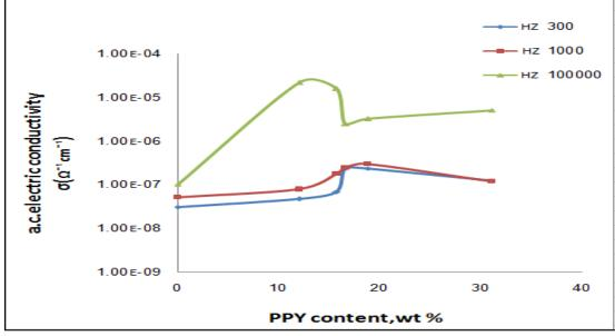
Figure(4):The dependence of total conductivity on polypyrrole content at (300,100 and 100000 Hz)
