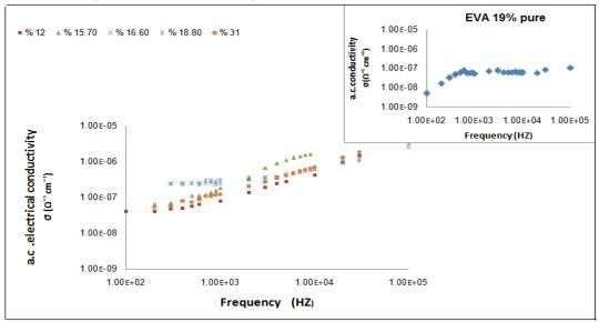
Figure(3):The frequency dependence of total conductivity for the pure EVA and its composites (with PPy) This is evident from Figure (4),wherein , the conductivity is plotted as a function of weight percent of PPy for some selected frequencies (300, 1000, and 100,000 Hz). Further almost all the blends show similar behavior up to
