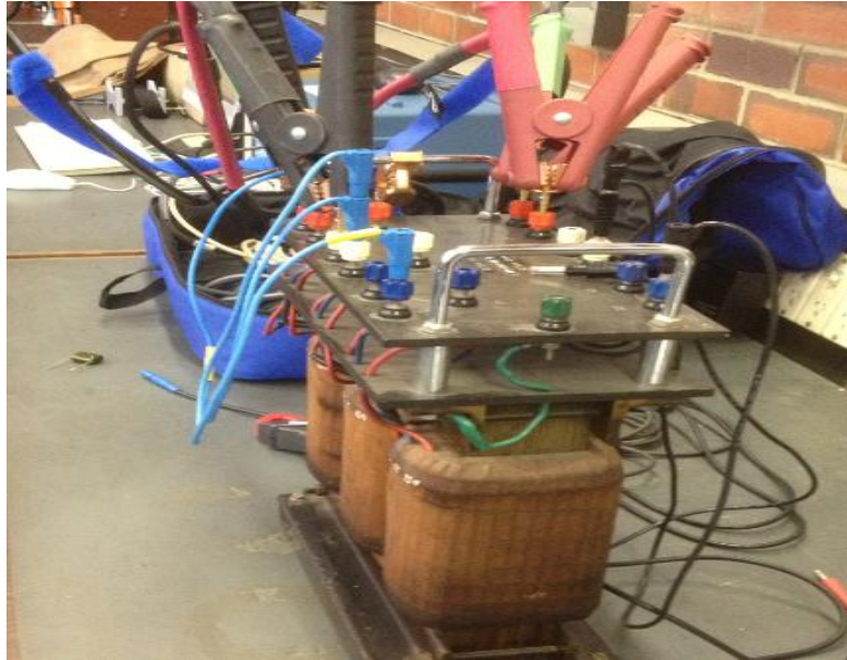
Fig.4.2 Case.2. Two SFRA laboratory experiment on a 440/55V 3-ph transformer.
