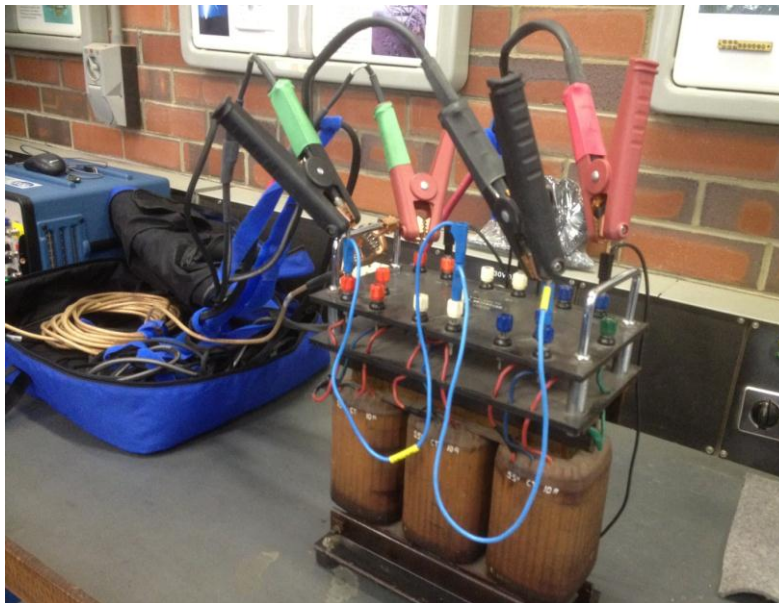
Fig.4.2 Case.2. Two SFRA laboratory experiment on a 440/55V 3-ph transformer.
