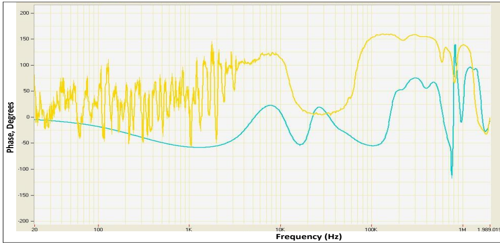
Fig.6.2 Two SFRA of a 440/55V 3-phase transformer (Frequency and phase).
