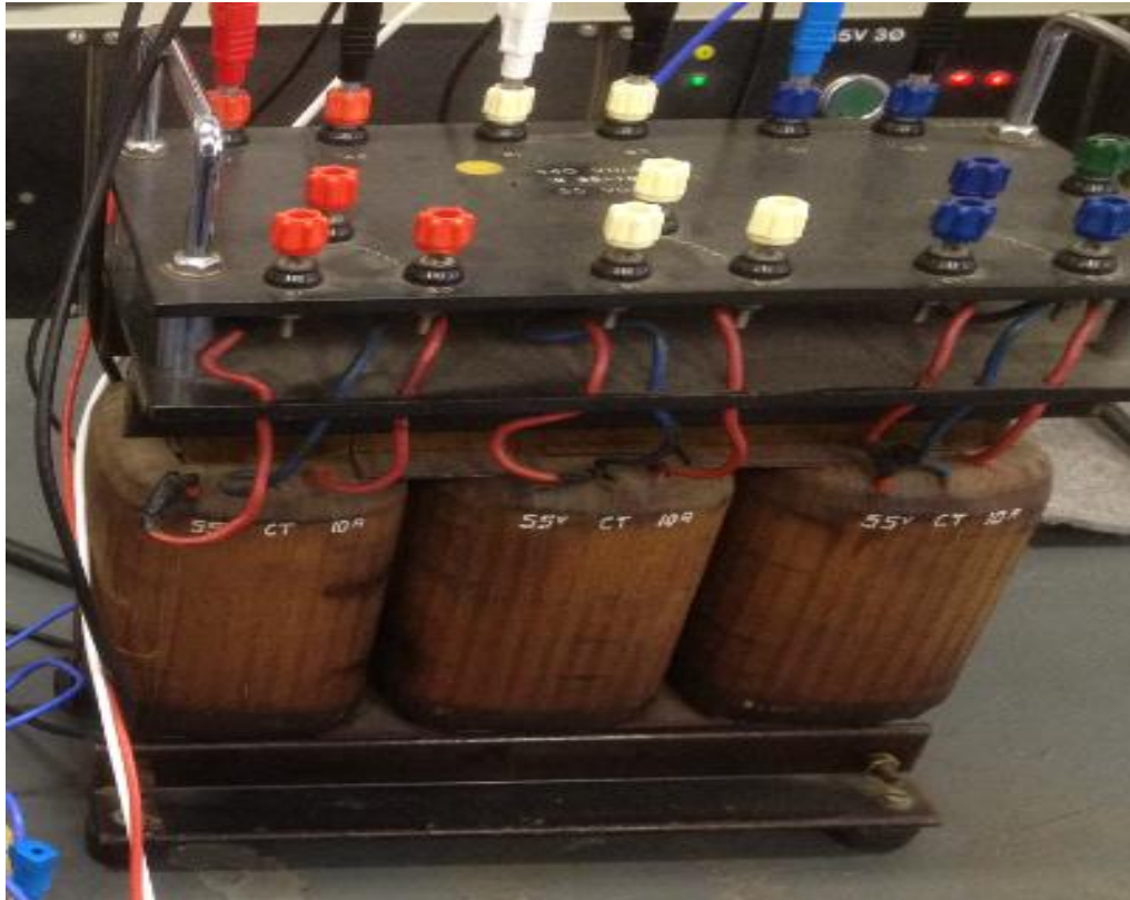
Fig.1 A 440/55V three phase transformer model used for the study (Curtin University Laboratory).
