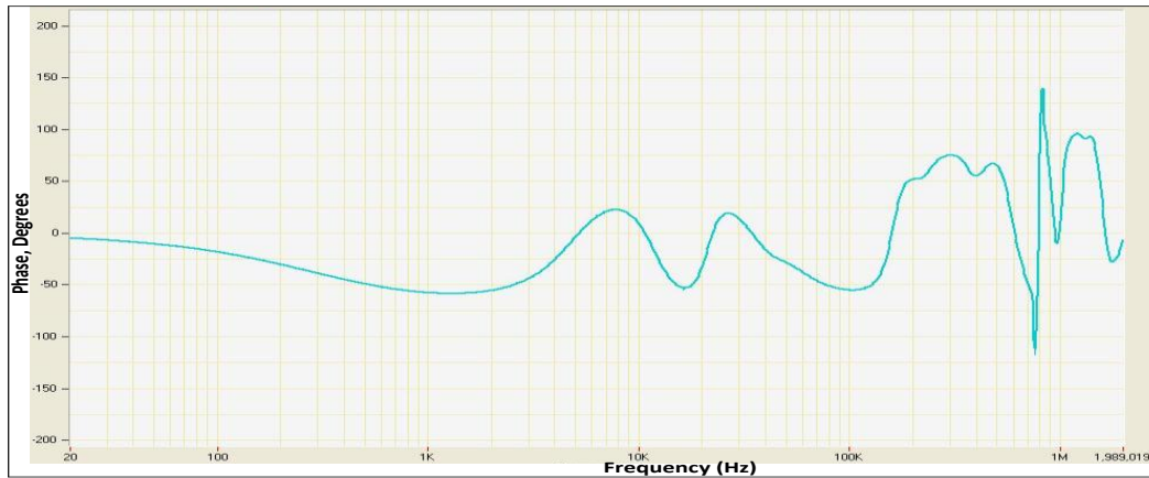
Fig.5.2 One SFRA of a 440/55V 3-phase transformer (Frequency and phase).
