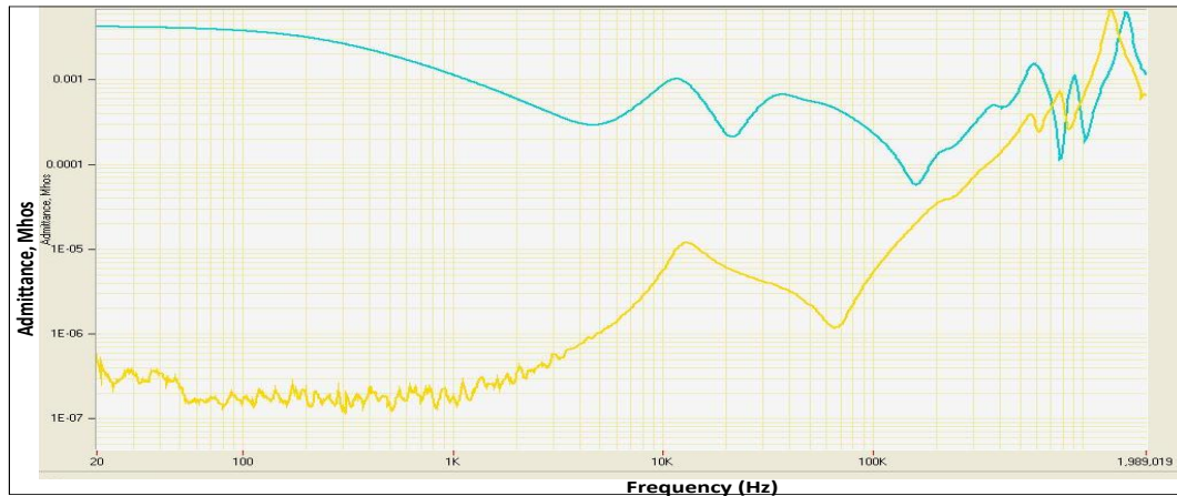
Fig.6.4 Two SFRA of a 440/55V 3-phase transformer (Frequency and admittance).
