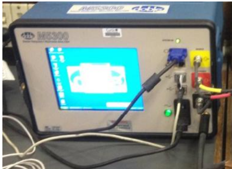
Fig.2 M5300 SFRA Analyser, Curtin University Laboratory.
