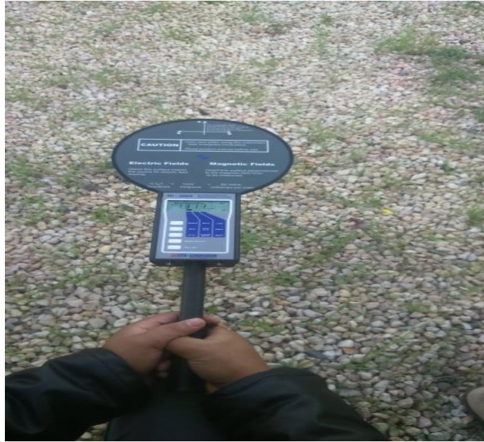
Figure (3.6) The device used for measurement (HI-3604)
