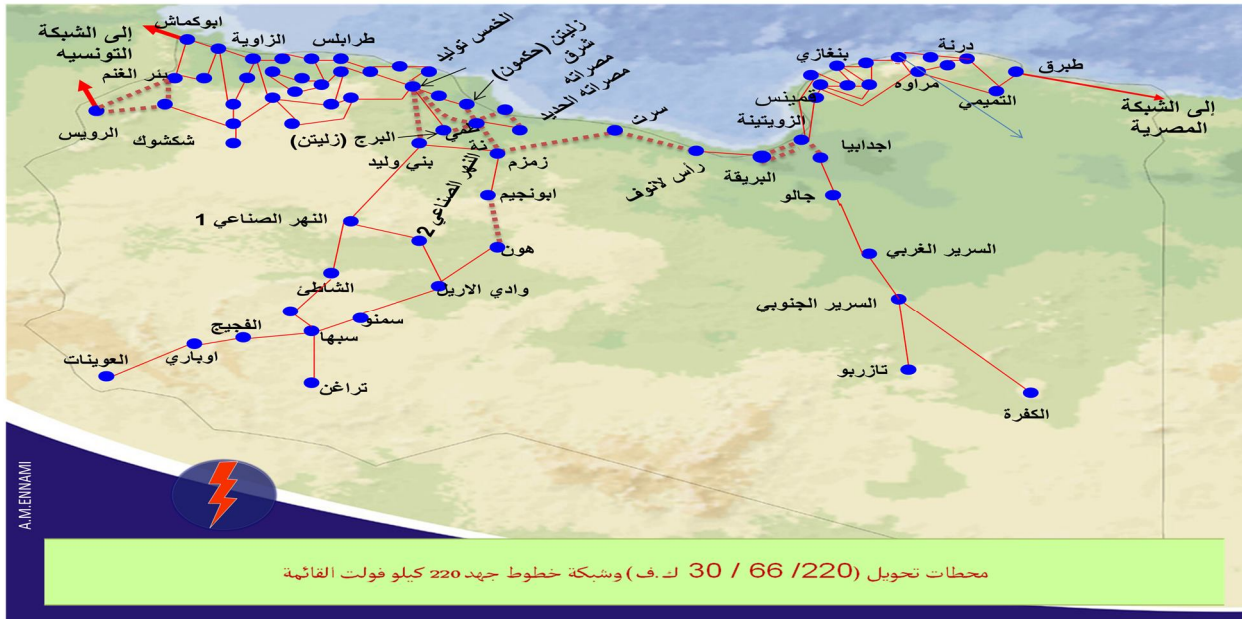
Figure (3-4) The transfer stations (220/66/30 kV) and the 220 kV distribution network in Libya
