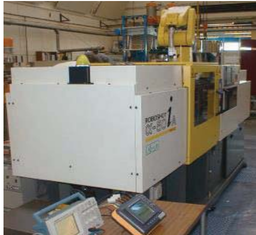
Fig 4. Injection moulding machine with gas assisted injection, Battenfeld beam robot, and Polymer Insights intelligent process monitoring, polymer engineering laboratory at Bradford University [9].
