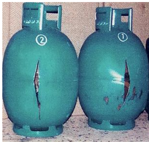
Fig.3. Failure Locations of the cylinders.
